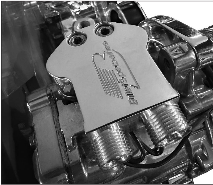
Figure 16: Install Compressor Manifold
